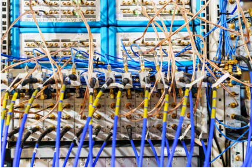
A stack of classical control electronics used to generate and measure electronic signals. Photo credits: Marc Blommaert for QuTech.
